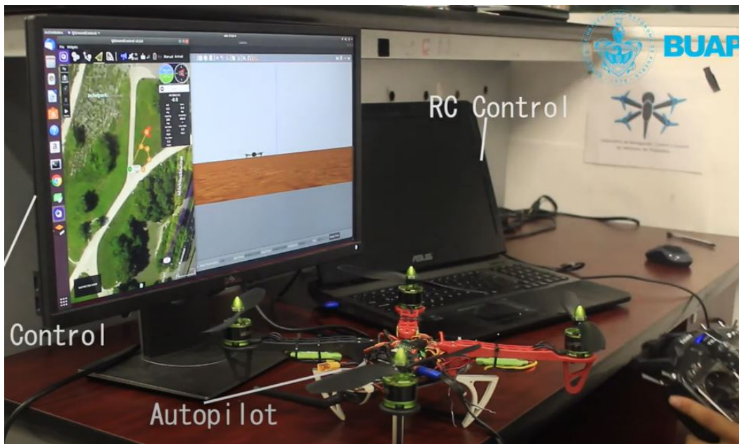
Fig. 6.3: Implementation of the Hardware in the Loop Platform.
