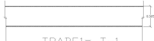
TRABE 1= T-1 PERFIL IPR 305 x 205mm 66.966 Kg/m
