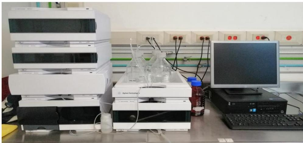
Figura (12). HPLC (1260, Agilent Technologies, Santa Clara, CA, USA)
