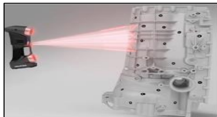
Figura 19 Levantamiento de targets, manual de Creaform Handy Scan 700
