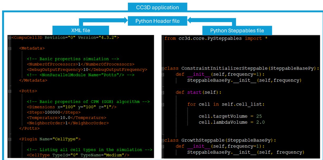
Figure 3.3 general structure of a CC3D application with an XML file, containing the general properties of the simulation, like lattice dimensions or cell types, and a Python stoppable file with specific biological processes are described such as the growth rate and cellular division conditions.
