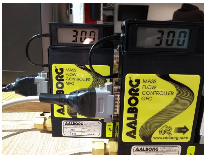
Figura 3.11: Flujómetros GFC Mass Flow Controllers.
