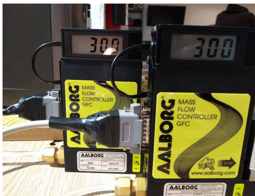
Figura 3.14. Flujometros GFC Mass Flow Controllers.
