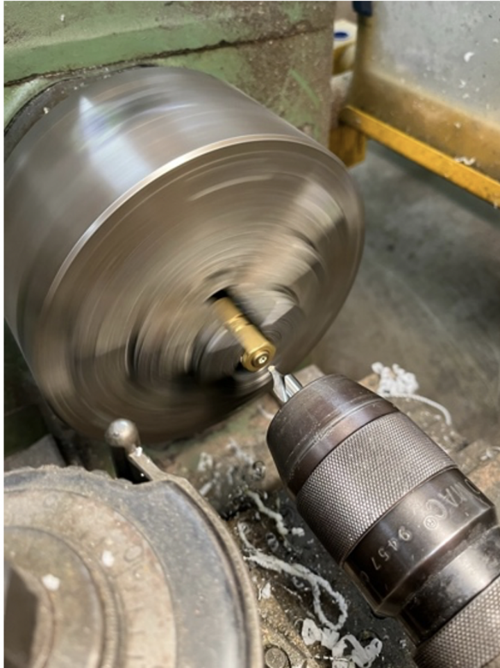
Figure A.4: A gas plug is being drilled to permit the passing of the wires.
