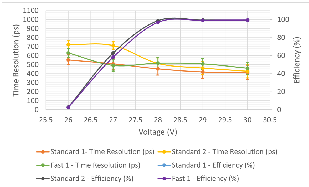
Figure 5.9: Results of the time resolution and efficiency of the detector configuration of BC-404 hexagonal plastic scintillator (thick) with a 6x6 mm SiPM on each side (TwoSiPMs) using the digitizer.
