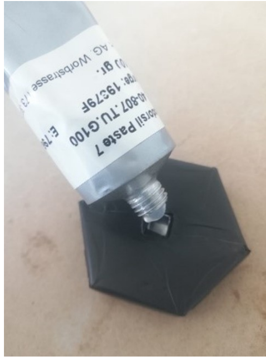
Figure 4.9: Rhodorsil paste 7 optical grease.
