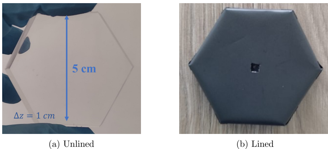
Figure 4.2: BC-404 Hexagonal Plastic Scintillator (New).
