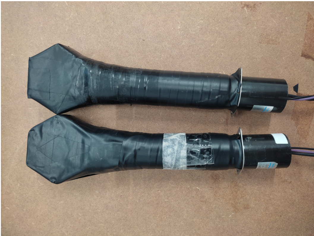
Figure 4.11: PMTs used as trigger for the SiPM characterization tests.
