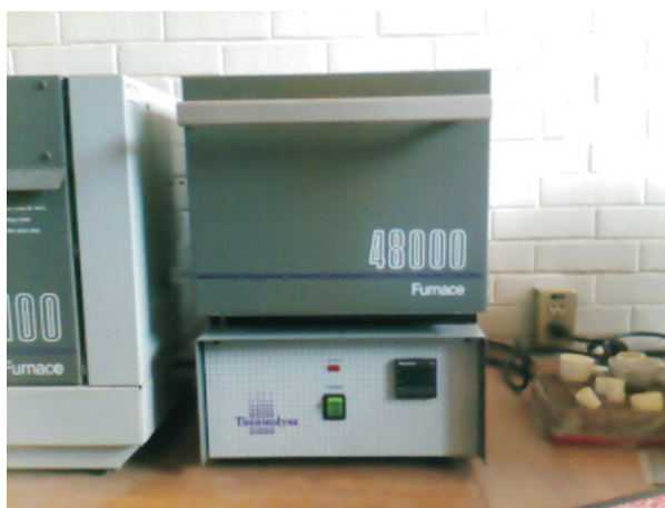
Figura 2.3: Mufla (Thermolyne \pm 4^\circ C )
