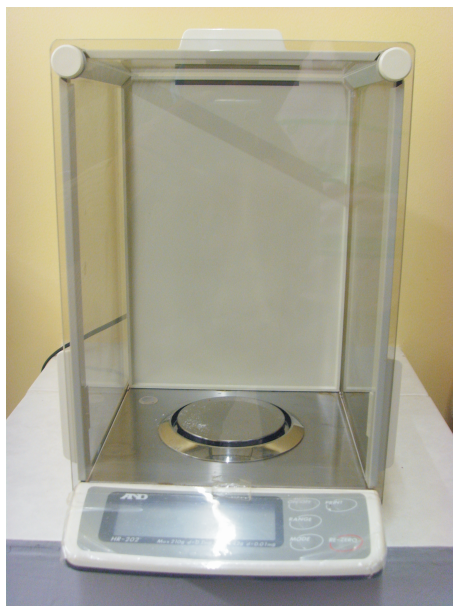
Figura 2.1: Balansa Analítica (Denver Instrument Company \pm 0.0003g )
