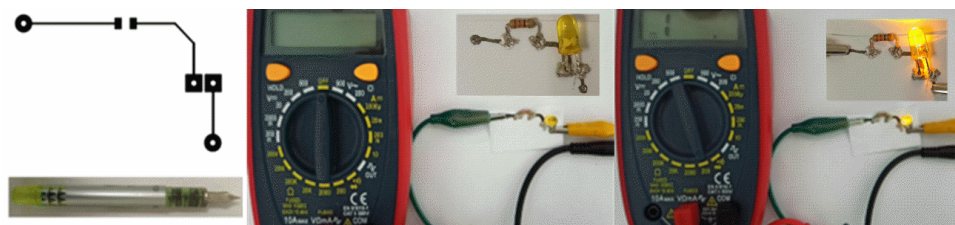
Figure 4.17. Design of drawing circuit with AgNPs ink with a fountain pen on photographic paper. Prototype to show a simple hybrid PCB.
