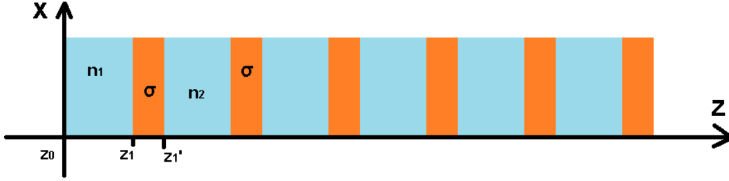
Figure 2.2: One-dimensional photonic crystal with a conducting two-dimensional material.
