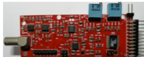
FIGURE 1. Front-end card to read out the APD and PMT detector signals.
