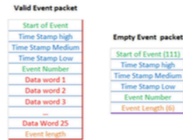
FIGURE 4. On the left, the data packet for a valid pulse and, on the right, the data packet for an empty event.
