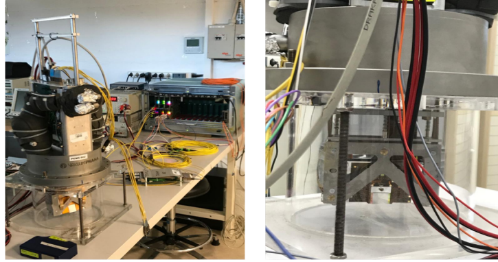
Figure 1.10: Silicon 3D Pixel Roman Pot. A picture taken during the tests on these devices is on the right, while a close-up photo is on the left. [39].
