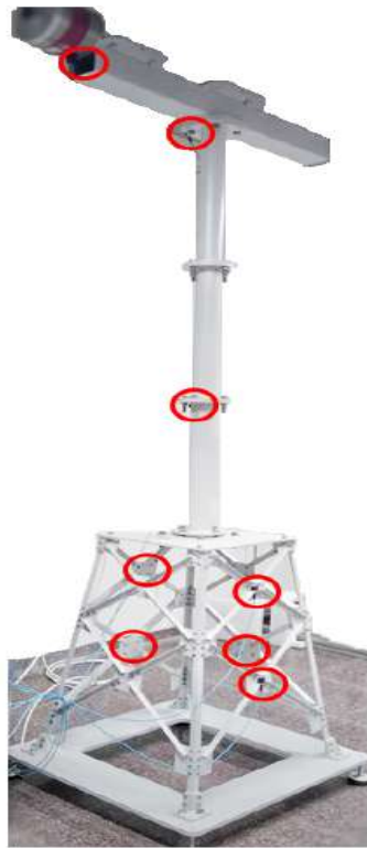
Figure 6. Location of the sensors on the overall structure.
