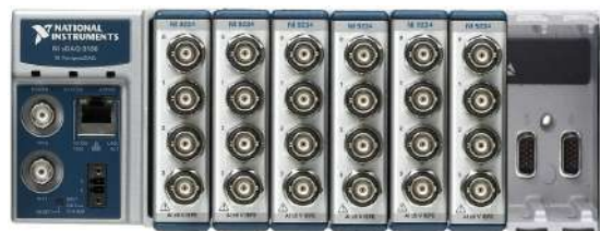
Figure 7. Data Acquisition System (DAQ) used in this work: cDAQ-9188 chassis and six NI-9234 modules from National Instruments.
