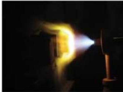
**Figura 3.** Photograph of the oxyacetylene ablation process.
