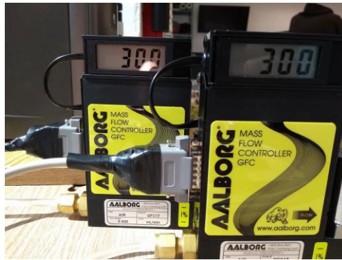
Figura 3.15: Flujómetros GFC Mass Flow Controllers.
